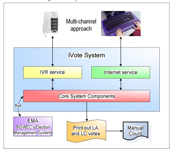
Figure 3 - iVote System Architecture Schematic
